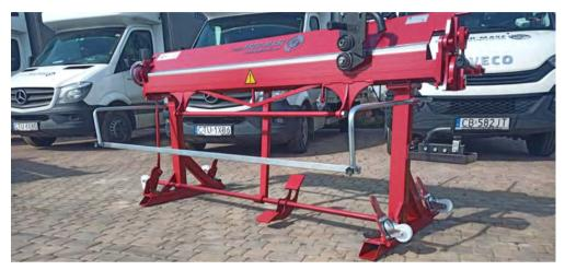
Both types of bending machines: both RED and RED Plus have an identical supporting structure. The difference between the two machines is that the RED version does not have a foot lever for raising and lowering the upper beam, while the machine has two side levers located on both sides of the machine.
