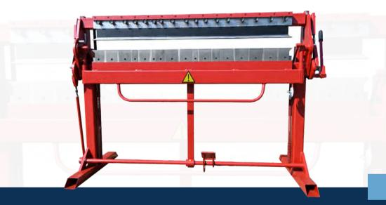
The SGR bending machine is equipped with segments in three beams, upper, lower, as well as in the bending beam. Sheets can be bent on all sides, producing complex shapes for boxes or elements bent up and down. A multi-purpose machine - a strong, heavy and very solid segment bending machine - this is not a typical bending machine - it is much stronger and more durable than other machines.
